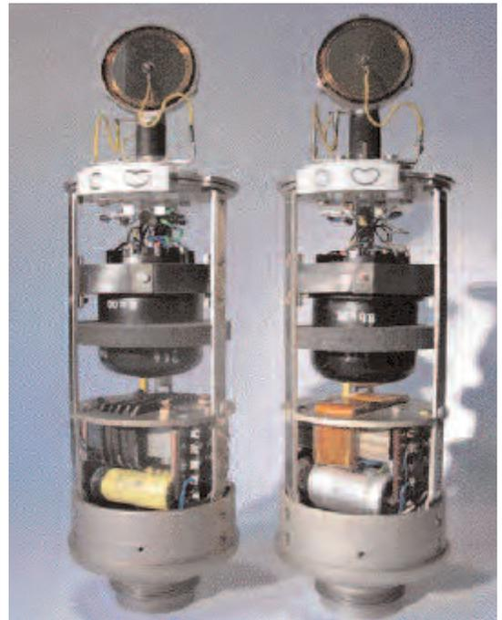
*The insides of Gunter's U47 (on the left) shows a remarkable likeness to an original Neumann. Many 'look-alikes' fail to impress on closer inspection of the internal electronics. The Wagner U47, however, is virtually identical to an original U47 shown on the right.*
